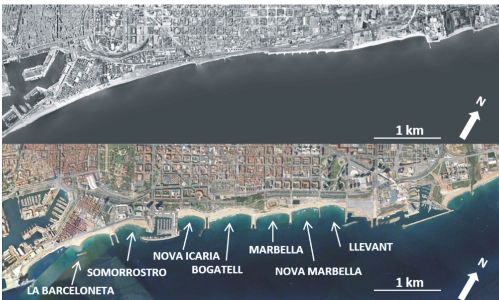
Fig. 1 - Comparison of the configuration of Barcelona city beaches in 1956 (above) and 2015 (below).
